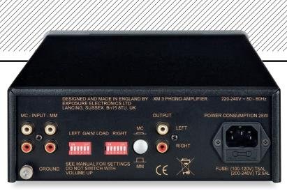
**ABOVE:** MM and MC inputs on RCAs are selected via a pushbutton while DIP switches select cartridge loading and gain from +40dB to +60dB
