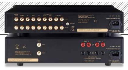
**ABOVE:** The 3510 pre [top] offers five line inputs (one for an MM/MC phono option), a tape loop and two preamp outs on RCAs. The 3510 power amp [bottom] includes RCA inputs and dual 4mm speaker cable sockets (for bi-wire applications) but are for banana plugs only, so there is no provision for bare wire or spades here
