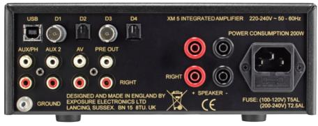
Plenty of connectivity, given the limited rear-panel real-estate. BNC sockets (D1, D3) accept S/PDIF digital for more accurate termination. Loudspeaker sockets accept 4mm plugs alone.
