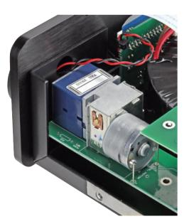
This motorised ALPS volume control is just one of the numerous audiophile-grade components that helps the XM5 work its musical magic. Note too the high-grade printed circuit board – which is made of fibre-glass, rather than the bonded-paper of cheaper products
