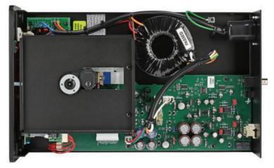
Despite its compact size the Exposure has a hefty linear power supply that contributes to its overall sound.
