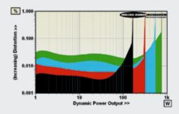
ABOVE: Dynamic power output versus distortion into 80hm (black trace), 40hm (red), 20hm (blue) and 10hm (green) speaker loads. Max. current is 27.6A
