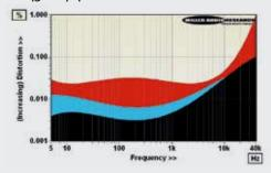
ABOVE: Distortion vs. frequency at 1W/80hm (black, 5Hz-40kHz), 10W (blue) and 70W (red, 20Hz-20kHz)
