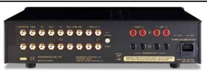
**ABOVE:** The 3510 offers five line inputs (one for an MM/MC phono option), a tape loop and two preamp outs. Dual 4mm speaker cable sockets support bi-wiring but are for banana plugs only – no bare wire or spade lugs here!
